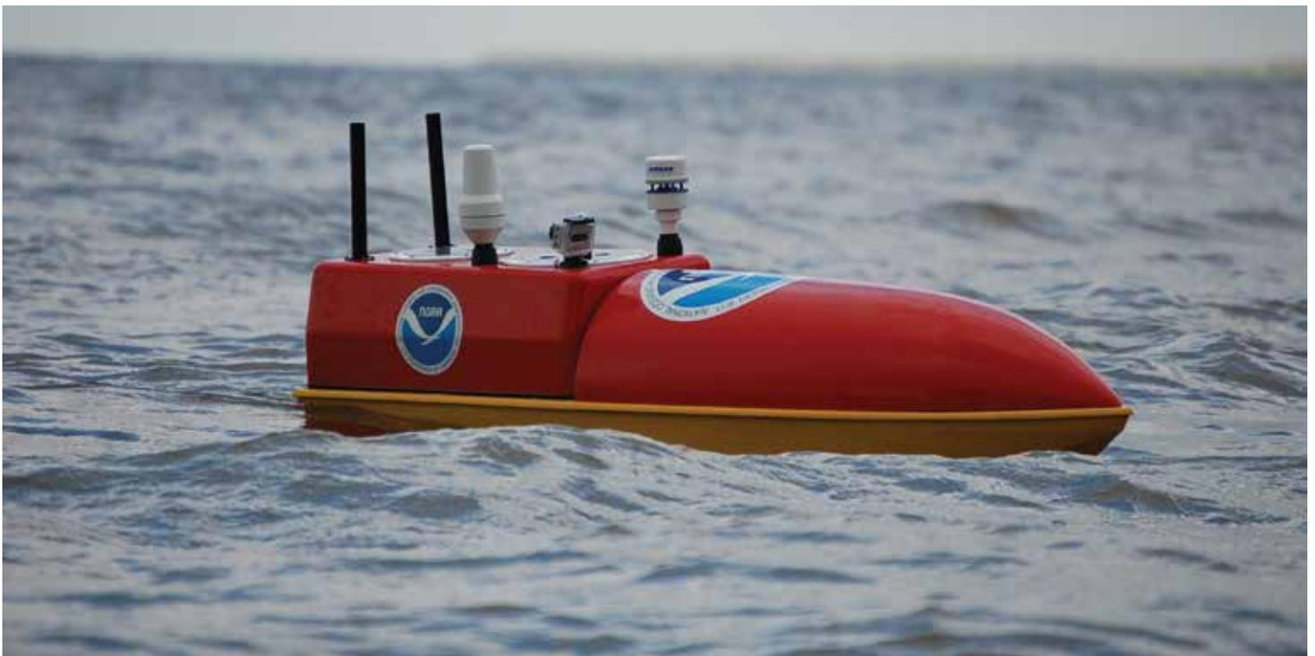
EMILY, a 65-inch water-tight craft, is one of NOAA's hurricane research platforms. Outfitted with a satellite link, camera, battery and gasoline motor, and a variety of sensors, EMILY will collect sea-level data from within a hurricane. *Credit: Hydronalix Inc.*
